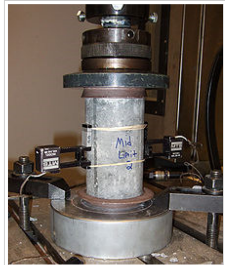
Compression testing of a concrete cylinder
