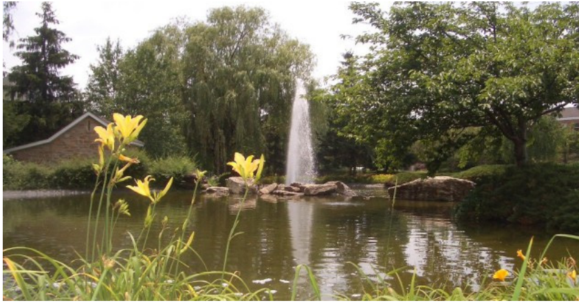
Retention (wet) basin made into an attractive landscape feature
