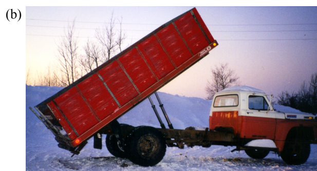
Hydraulic cylinders in a dump truck
